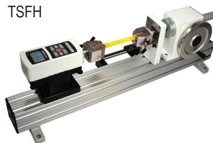
The TSF is shown testing a compression spring, with a Series 5 digital force gauge and digital travel display
