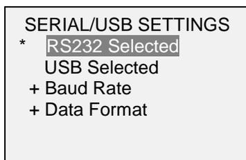
Select either RS-232 or USB input (output is always active for both the USB and RS-232 ports). Communication settings are permanently set to the following:
