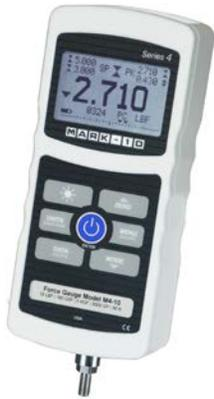
Thank you for purchasing a Mark-10 Series 4 digital force gauge, designed for tension and compression force testing applications from 0.12 lb to 500 lb (0.5 N to 2,500 N) full scale. The Series 4 is an essential component of a force testing system, typically also comprising a test stand, grips, and data collection software.
