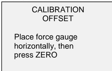
5. Place the force gauge horizontally on a level surface free from vibration, then press **ZERO**. The gauge will calculate internal offsets, and the display appears as follows:
