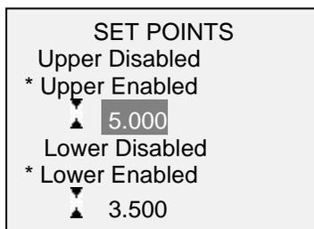
Either one, two, or none of the set points may be enabled. To toggle between the tension and compression directions, press the **DIRECTION** key.
