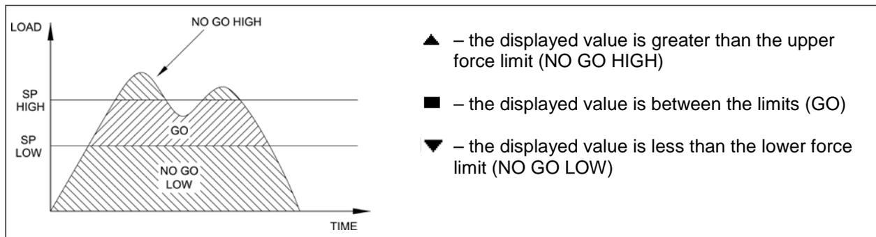
**Note:** Set point indicators and outputs reference the displayed reading, not necessarily the current live load.
