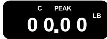
To TARE, affix the required adapter or fixture to the gauge. Orient the gauge so that it is positioned as it will be during testing. Depress the ZERO key to tare the gauge.
