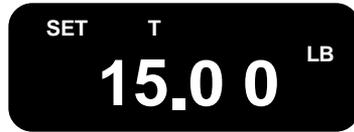
To set the LOW LIMIT (T), depress **SET**. The low limit will be displayed. The SET icon will be displayed along with the "T" indicating that you are in the setup mode for LOW LIMIT.
