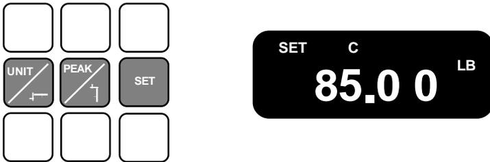
To set the HIGH LIMIT (C), depress **SET**. The high limit will be displayed. The SET icon will also be displayed along with the "C" indicating that you are in the setup mode for HIGH LIMIT.
