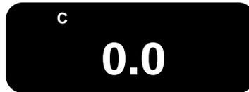
To display the **NO LOAD ZERO**, depress the ZERO key. The gauge will display the no load zero measured during the previous and most current calibration. The display will indicate the no load zero reading in % of A/D range).
