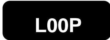
Depress the ZERO key and the gauge will transmit an ASCII character "U" (See Section X.X Data Collect Mode) back to itself via an RS232 loopback connector (Not included). Depress ZERO again to exit the loopback test.
