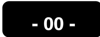
Place the gauge on its back side in a horizontal position, depress the ZERO key. The gauge will display a blinking "-00-" then display the applied force in % of A/D range until ZERO is depressed again.
