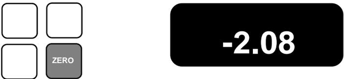
To display the **SOFTWARE REVISION NUMBER** used with the gauge, depress the ZERO key. The gauge will display the revision number, e.g. Revision 2.08.
