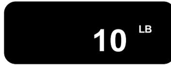
To display the **CAPACITY** and **UNITS** used with the gauge, depress the ZERO key. The gauge will display the capacity and units used in the previous and most current calibration.
