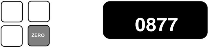
To display the **SOFTWARE PART NUMBER** used with the gauge, depress the ZERO key. A four digit number will appear representing the software part number.
