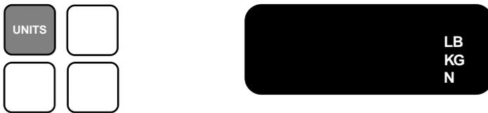
With gauge power ON, depress the **UNITS** key to cycle through available force measurement units (LB, KG, N). Release the key when the desired unit is displayed.
