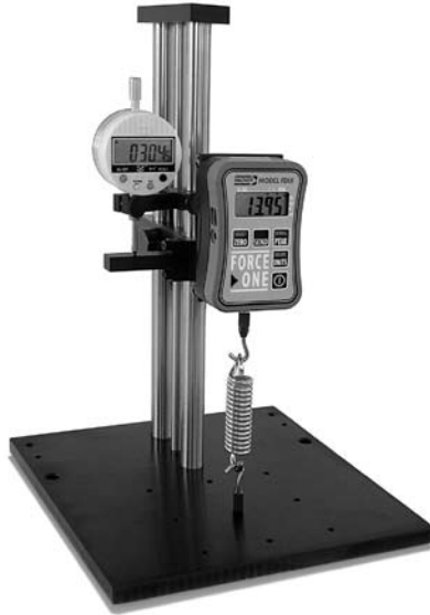
Force One™ FDX shown mounted on Wagner FTK 100 Test Stand
