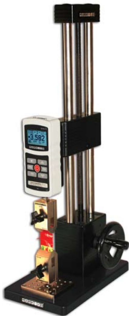
ES30 Manual Handwheel Test Stand
